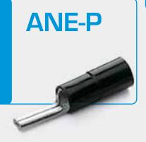
ANE-P series terminals are made from electrolytic copper, rolled, tin plated and brazed. The interior of the PA6.6 insulation sleeve is funnel shaped so as to ensure complete and easy introduction of the conductor strands.
