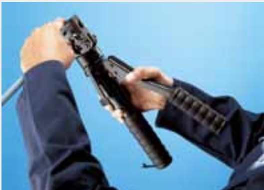
The operator can advance the dies using only one hand, leaving the other hand free to position the connector.
