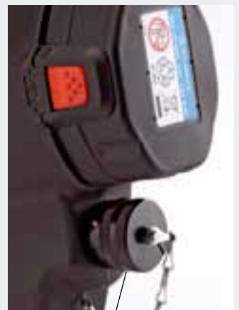
Socket for 12-14.4 V dc external power supply
